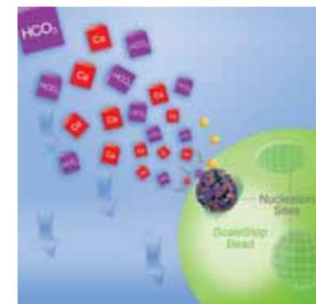
Once the crystals grow to a certain size they are released from the bead. The crystals in solution keep the hardness out of the water so that it can't deposit and form scale on the plumbing surfaces or interfere with soaps and detergents.
